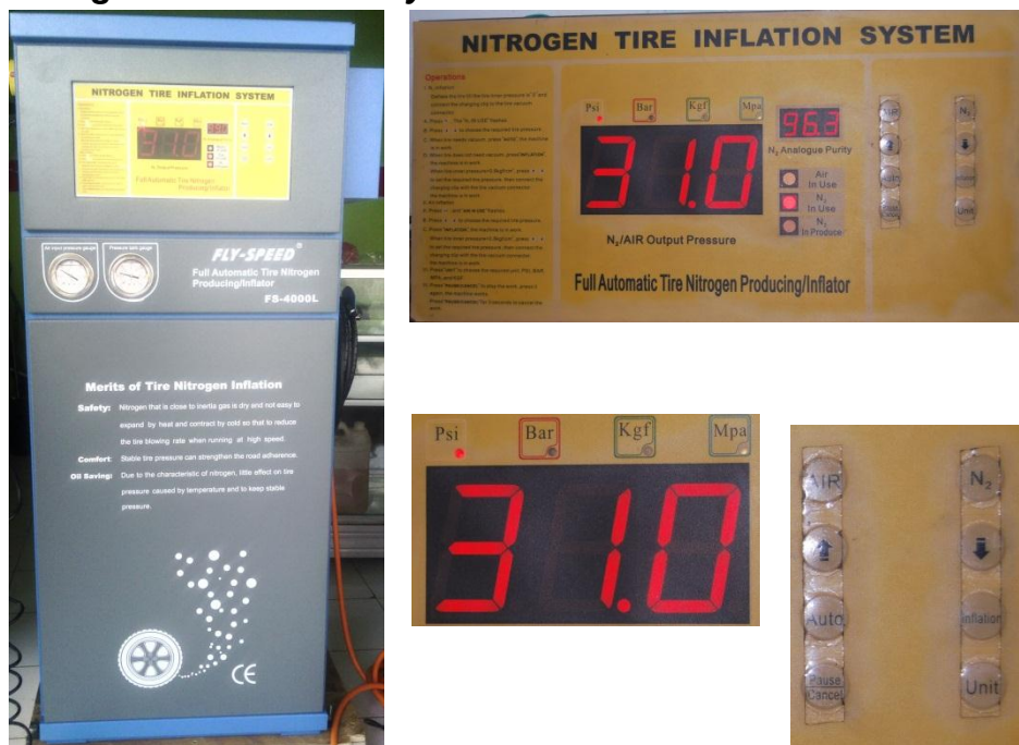
Gambar 2.1 Nitrogen tire inflation system
